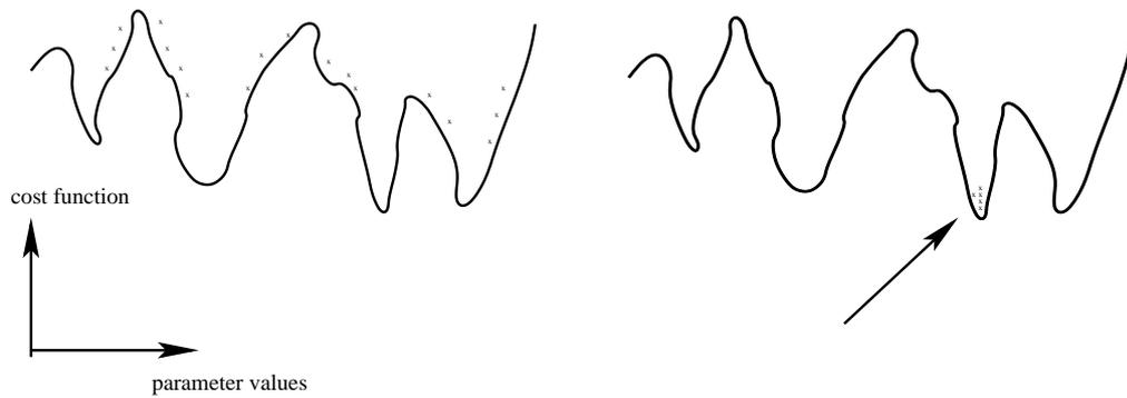
Figure 14: The cost function landscape, and the behaviour of a classical global optimization algorithm such as simulated annealing, which normally tries to find the global optimum.
