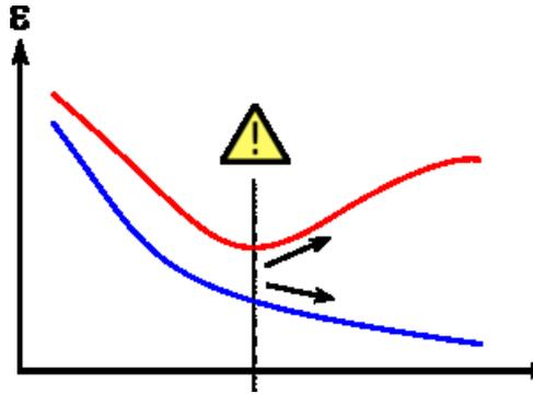
Figure 11: The blue curve is the increasing agreement to estimation data, with increasing model complexity (i.e., flexibility). The red curve shows that there comes a point where the agreement with new validation data gets worse. This is the problem of over-fitting.
