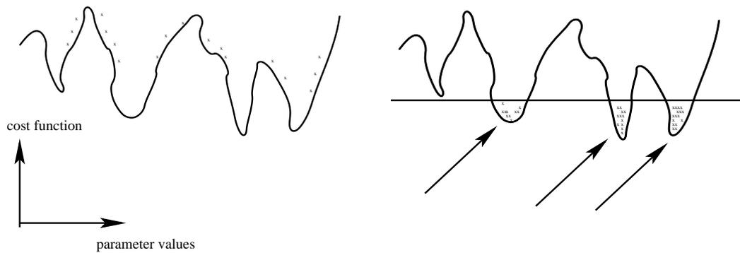
Figure 15: The cost function landscape, and the behaviour of a modified global optimization algorithm, which seeks to identify a good approximation of the entire space of acceptable parameters.
